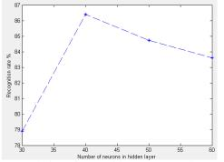
Fig. 5: Evolution of recognition rate according to the number of neurons in the hidden layer
